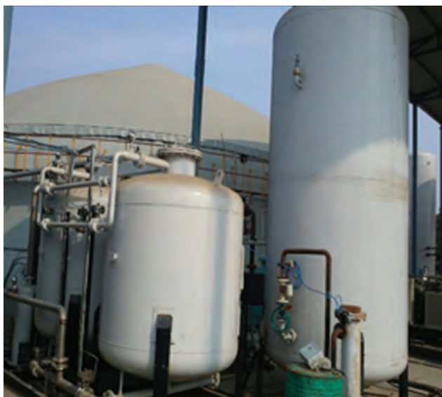
Fig. 2.33Purification through Vacuum Pressure Swing Adsorption System
